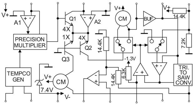
There are four building blocks in the AS3340 that affect the 1V/Oct tuning. Note that naming conventions for resistors and currents are taken from the AS3340 datasheet.
